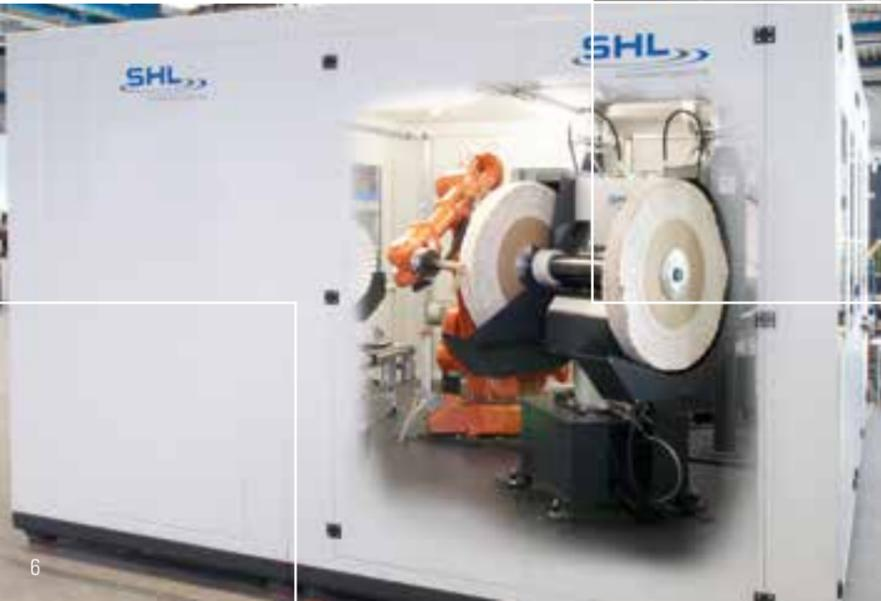
**Fig. 3** Polishing of fixtures
